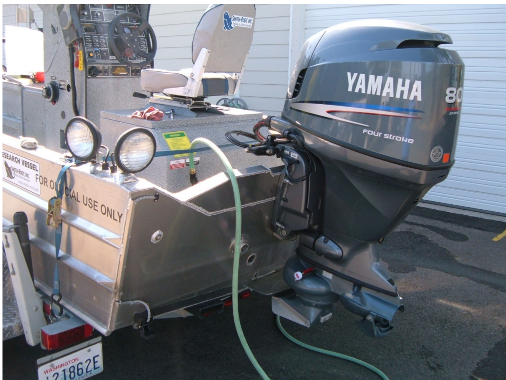
3D. Generator flushing adapter is attached. Ready to turn on water supply and flush generator and washdown pump systems.
