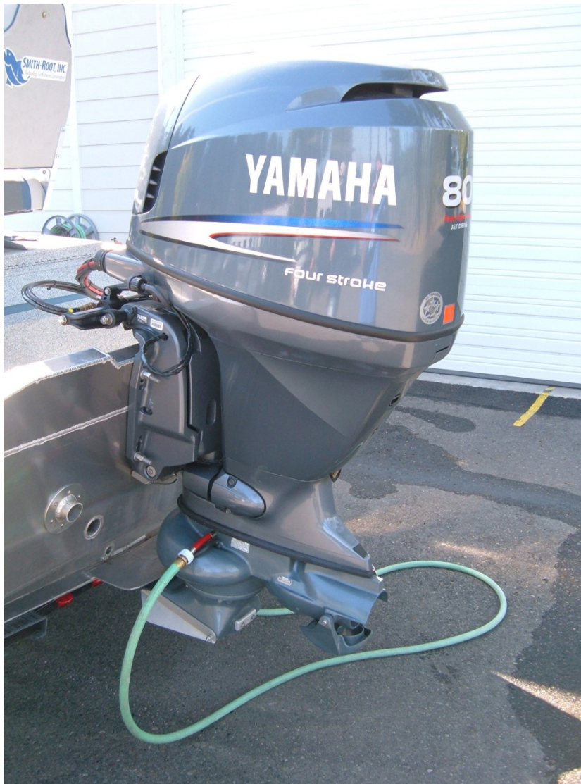
2C. Outboard flushing adapter attached to lower jet unit. Ready to turn on water supply and flush outboard system.
