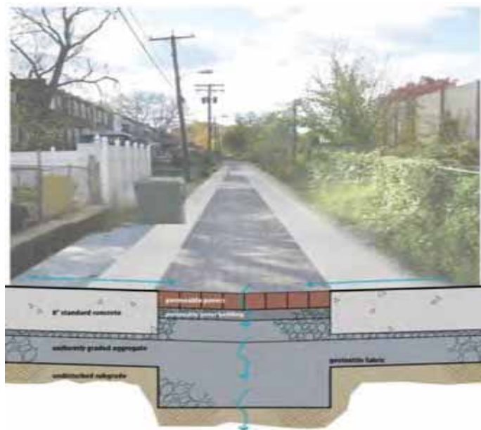
Typical green alley cross-section
