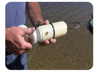
C.L.A.M.s weigh just over one pound, including the 4 AA batteries, and many can be easily taken to remote areas and left unattended to sample continuously for up to 36 hours at submerged depths up to 50 feet in marine or fresh waters.
