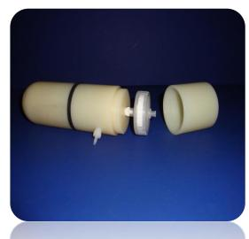
The C.L.A.M. (Continuous Low -Level Aquatic **Monitoring**) was developed to produce this unique extract. The **C.L.A.M.** is a small submersible extraction sampler, using EPA approved methodology **3535**, utilizing **SPE** (Solid Phase Extraction) media disks to sequester Pesticides, Herbicides, PAH's, TPH, and other trace organics from water.
