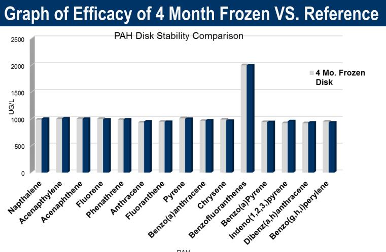
The acceptable RPD efficacy compared to the reference shows that the deployed disk can be stored in a frozen state for months without analyte degradation. Stopping the holding time clock for this method of sampling provides laboratories sample scheduling flexibility in peak times saving time and materials
