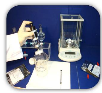
The **C.L.A.M.** uses field hardened encasements to actively draw a known volume of water through the SPE media during the extraction event. All the SPE media types are supported in custom housings which incorporate inlet flow dispersion, triple lofted glass pre-filters, supporting filters, and inert screens to field harden and reduce clogging.
