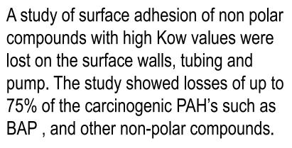
Sub-set sampling as done today, is providing samples to the environmental laboratory that are **biased low** for most all non-polar target analytes, simply because the holding container can't be solvent rinsed into the sub-set bottles.
