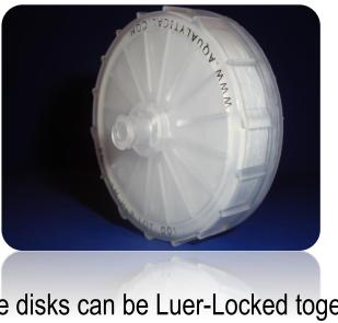
The disks can be Luer-Locked together to provide a multi-stage system for total and dissolved studies, varied media stages or breakthrough studies. The disks are also supplied with Luer plugs which can seal the disks after conditioning or deployment for secure transportation.
