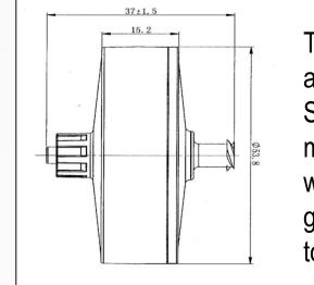
•Disk encasements are manufactured using high density polypropylene (HDPP) •The disposable SPE extraction cartridges, disks and syringes used in the laboratory for over 15 years are made of the same HDPP •The disks interior design uses HDPP media supporting screens, dispersion baffles, and glass pre-filtration filters to ensure an inert environment.
