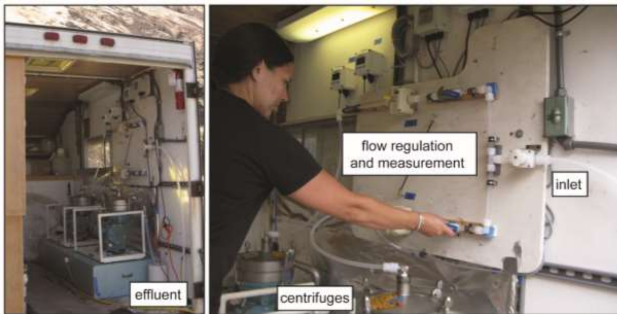
Figure 6: Centrifuge trailer and the flow control board for each centrifuge (right).
