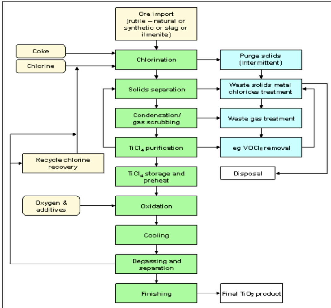
Figure 2. Outline flow diagram – titanium dioxide production by the chloride process route (European Commission 2007)
