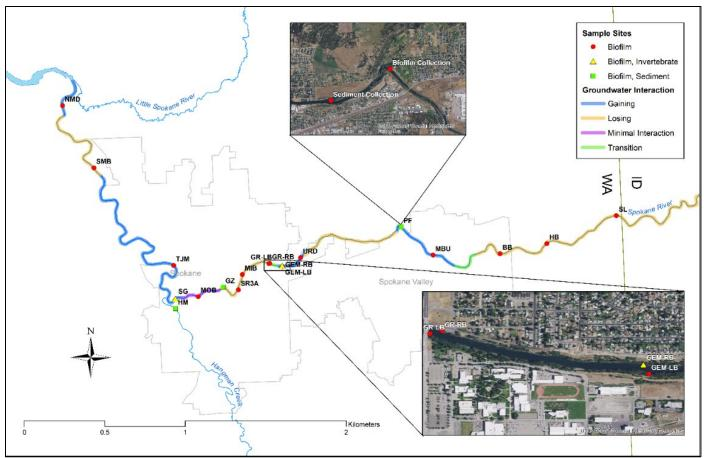
Figure 1. Map of the Spokane River showing sampling locations during the 2018 field study. Except for three sites (GR-RB, HM, SMB), the 2018 sampling sites will be resampled in 2019 (Figure 4, Table 7).
