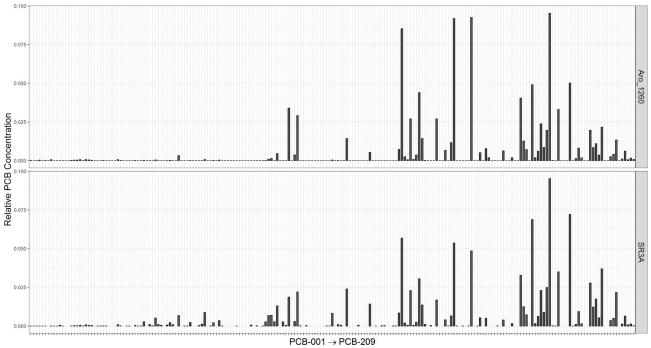
Figure 3. Relative PCB congener concentrations (PCB Congener/Total PCB) for unweathered Aroclor 1260 (top) compared to biofilm collected at site SR3A (bottom). The bars represent each PCB congener, ordered from PCB-001 (left) to PCB-209 (right).
