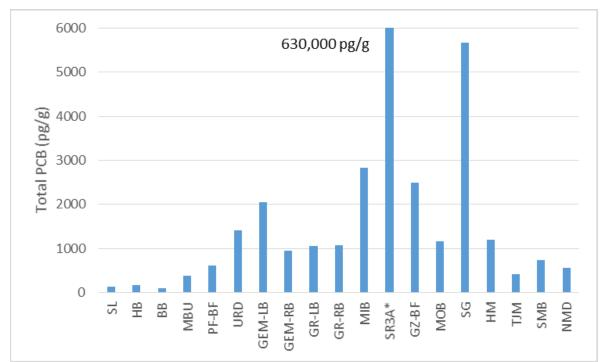
Figure 2. Total PCB concentrations measured in biofilms collected at sites in the Spokane River in 2018. Sites are ordered from upstream (left) to downstream (right). \*Site SR3A had a concentration of 630,000 pg/g and is off the scale of this plot.
