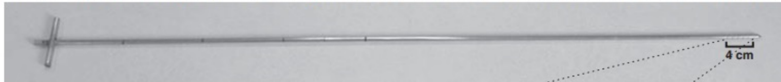
A. Pushpoint sampler. Rod lengths used were 91 centimeters and 183 centimeters.
