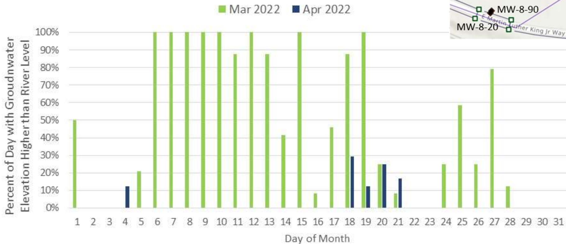
MW2-20 Continuous Monitoring Flow Reversal Events
