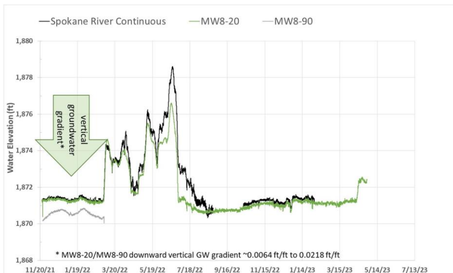
Figure 15. Graph of continuous groundwater level monitoring data for clustered wells MW8-20 and MW8-90, showing a consistent downward vertical gradient for the period late November 2021 through March 2, 2022.
